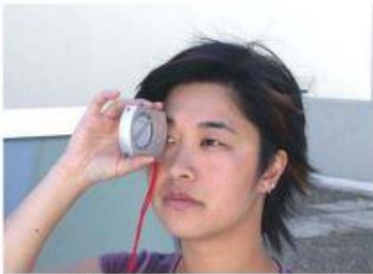
Figure 2: Both eyes open and clinometer vertical
