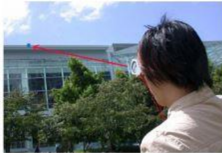
Figure 3: Sighting a point along top of building
