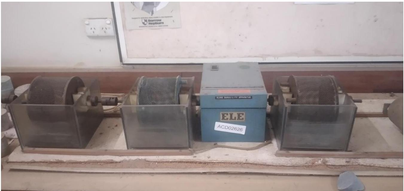
1. To set up to conduct the slake durability test, first you'll take the drum to weigh it and record its weight. We can only work with samples between 450 – 500 grams.
