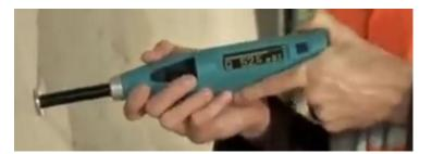
4. Fires and it records a Q value in this case it is 61.5 \_ This is, primarily a means of testing the hammer's log for rating
