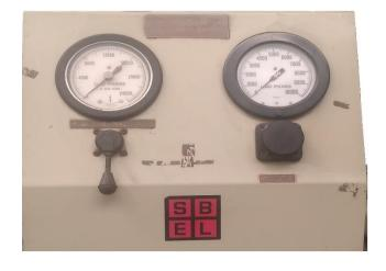
**3.** Now remove the Axial load pump and the Shear load pumps pins and free the handles to start pumping to apply load in the Axial and the Shear direction
