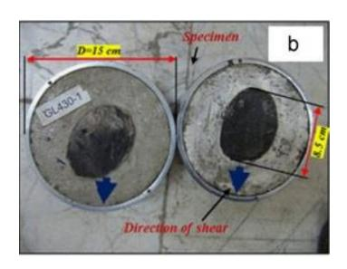
8. The cement paste must be filled up to the brim of the cells with the contacting surfaces of the discontinuity plane protruding out enough to make contact when the cells are clamped together.
