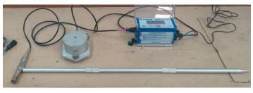
Open the glass cover of the vibration monitor control by releasing the 2 pin clips on the sides, ready to start and operate.
