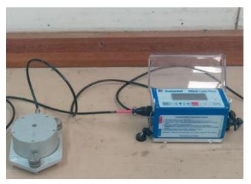
4. Assemble the prob shafts and connect them to extend the shaft and then connect the geophone and clip it to the clamp on the prob shaft. Pin it into the surface, have it standing upright
